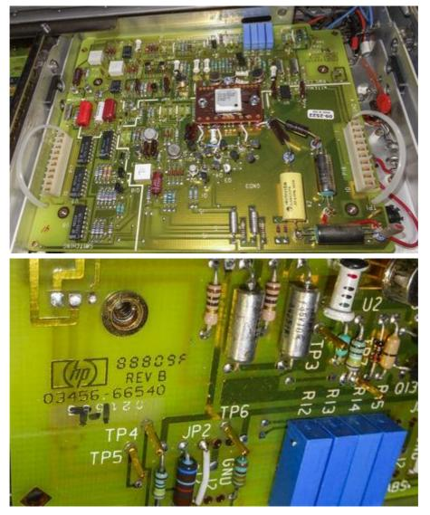
Analog circuitry domain implements various precision resistors and hybrids, which help to maintain high performance and stability of critical circuits.
