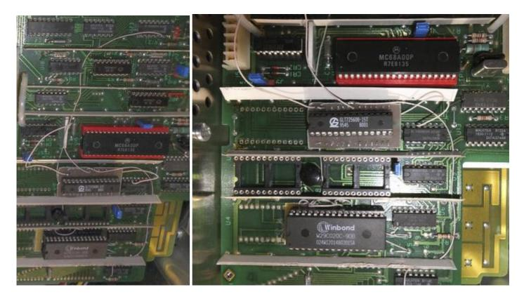
Everything else is similar to ROM repair workflow – careful removing old RAM chips from A4 PCB, soldering some socket pins with copper studs into PCB, so pin 14 of socket match PCB's pin 12. Ground to ground, data bus signals to data bus.
