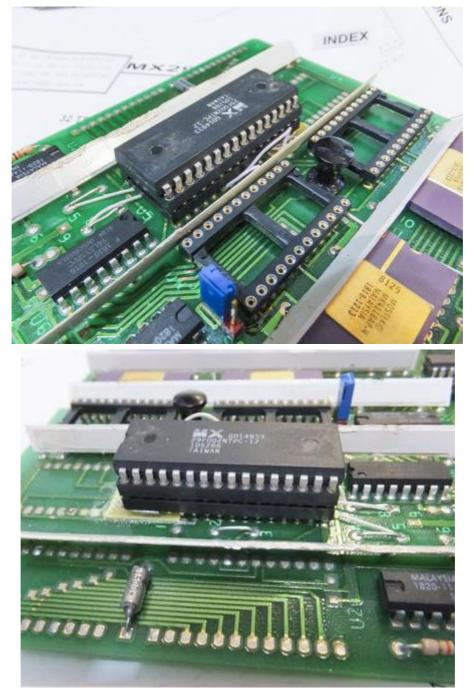
You can also spot second IC socket on photo. This is due simple reason, as my MX29F002 had missing data pin, so had to fix with extra bit. To avoid damage of socket mounted on PCB, this intermediate socket was used to hold fixed ROM chip.
