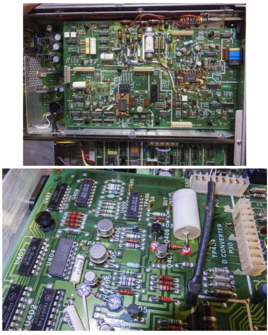
All analog inguard domain, including switching and A/D conversion parts, are controlled by inguard-controller, which is called so due to location in guarded faraday cage, isolated from rest of chassis and mains circuitry.
