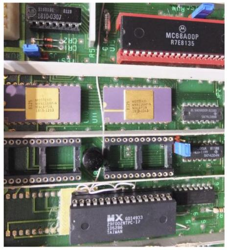
Now, after RAM replacement, instrument finally came back to life. Self-test discovered inguard-controller failure. In my case processor i8048 was installed in socket. Chip temperature was OK, so I just removed chip and installed back in. Immediately instrument went to normal operation and show few counts on display. So I went ahead and replaced old socket with modern high-quality collet-type socket. HP in **3456A-13A Service note** recommends to solder chip down to PCB.
