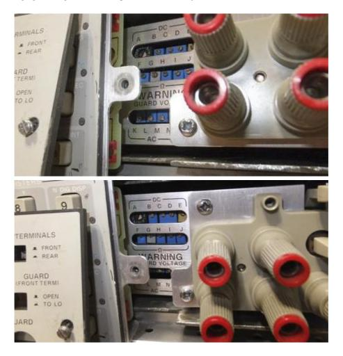
Good side of HP3456A – lack of NVRAM memories, and their battery cells. So calibration of 3456A cannot be lost due to longtime storage and battery depletion, unlike other instruments designed in 90's.
