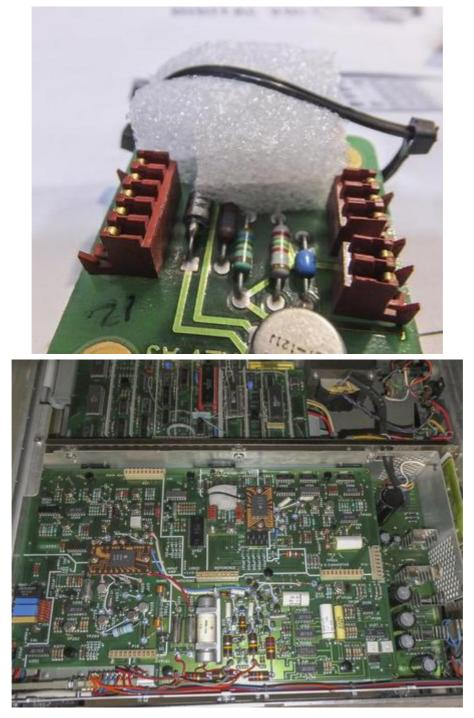
It's critical to be extremely careful, not to track tiny traces around or damage components. To further isolate reference there were foam caps installed on top and bottom surfaces of reference board, like was shown on photographs. It's best to fix these caps with simple fabric thread, instead of plastic coupler, as excessive pressure and mechanical force will cause extra stress to zener chip and output voltage will observe larger drifts.
