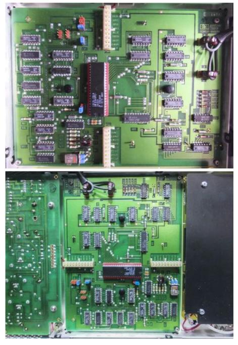
This controller receiving commands of operation mode, (ACV, DCV, Ohm or RATIO measurement) and type of operation (such as autorange/manual range, integration time, resolution, autozero functions and filtering) via isolation transformers interface with main outguard processor/controller. This is interesting implementation, as modern instruments usually use optocouplers for similar isolation task.
