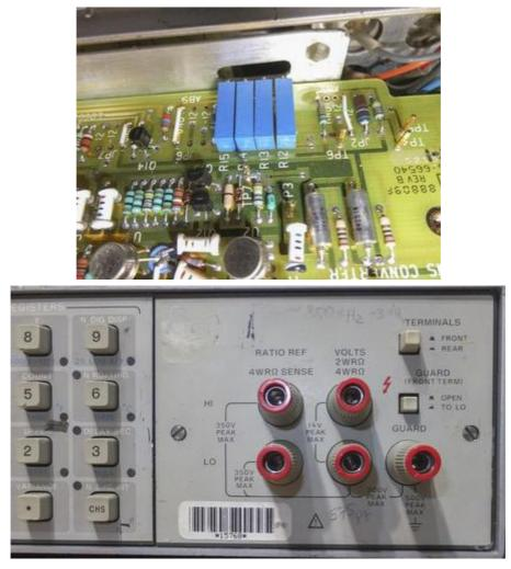
Cover should be installed back after calibration operation to maintain stable thermal profile.
