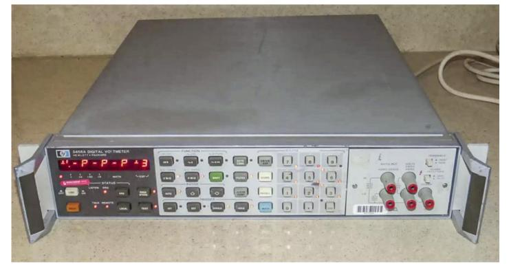
After arrival unit was switched for proper mains voltage (220VAC here), prior to connecting power. First attempt to boot meter revealed random front panel operation, without any system or pattern. Most of keypresses do not change any behavior, and some cause random indication changes.
