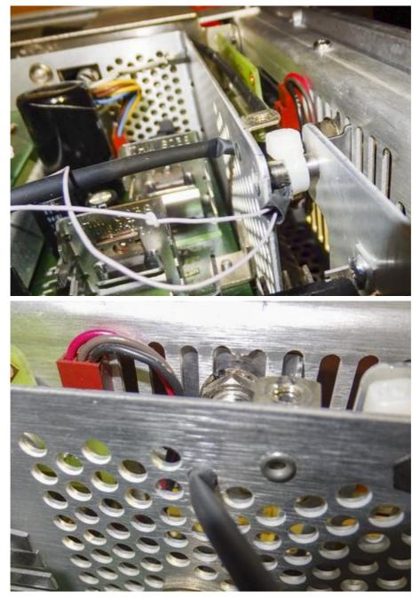
Thermal sensor wiring was routed using existing holes and areas, as you can see from provided photos.
